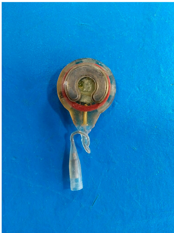
Figure 8 Explanted receiver from revision surgery of a “twiddler” (Note the entangled wire).
