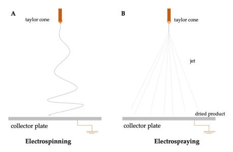
Figure 5. Schematic illustration of the basic setup for (A) electrospinning and (B) electrospraying.
