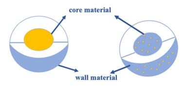
Microencapsulation is a production process of small structures produced by polymeric walls that surround bioactive compounds (Figure 1) [3,4].
