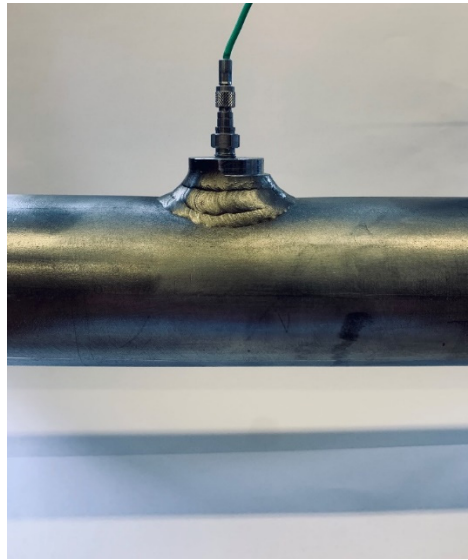
Figure 2. Closer view of the installed side-wall pressure sensor.
