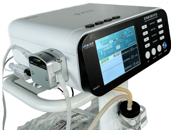
Fig. 1 The patented perfusion and suctioning platform with pressure feedback and control function
