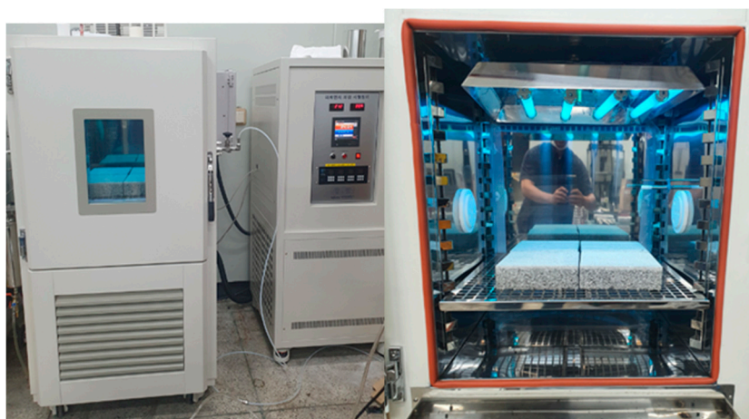
Figure 7. Laboratory experiment with environment chamber.
