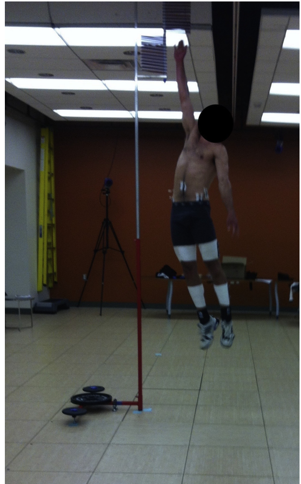
Fig 2. Demonstration of peak vertical jump following a 3-step spike approach. Vertical jump height is measured by Vertec device (left) as well as reflective markers attached to participant's midsection using video motion analysis.
