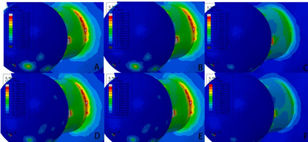
**Fig. 4.** Von Mises stress distribution of the attachment. A, B, C correspond to the conventional zirconia group, the ultra-translucent zirconia group, and the PEEK group of design 1 respectively. D, E, F correspond to the conventional zirconia group, the ultra-translucent zirconia group, and the PEEK group of design 2 respectively.
