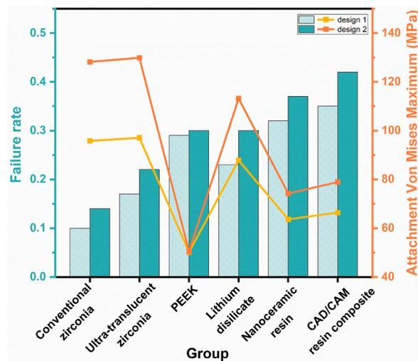
Fig. 6. Comparison of failure rate and maximum stress of the attachment junction.
