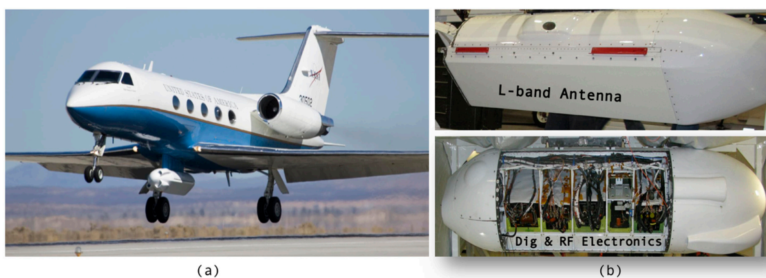
Figure 1. (a) UAVSAR platform with instrument pod located below the fuselage. (b) UAVSAR instrument.
