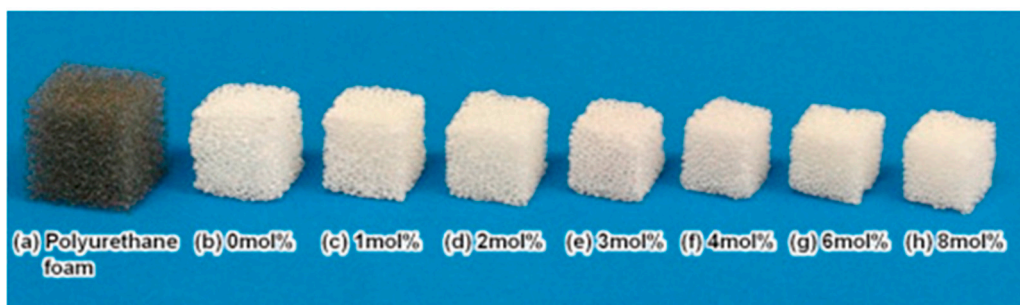
Figure 8. Typical macroscopic structure of: (a) the polyurethane foam template and (b–h) TCP foams prepared with calcium phosphate slurries containing different amounts of MgO. Reprinted from [122] with permission from Elsevier.
