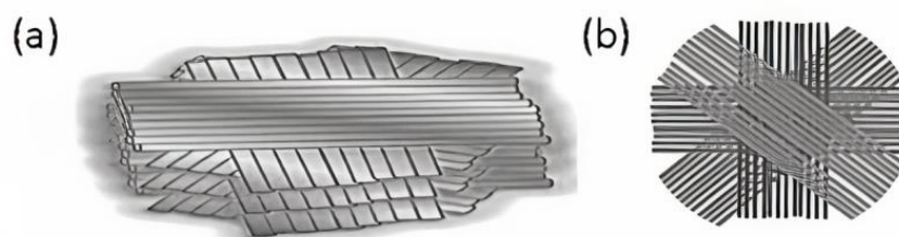
Figure 1. Schematic illustration of the multilayered composite (a) consisting of layers with 3D-architected helicoidally aligned fibers; (b) with fiber alignments of [0°, 45°, 90°, 135°, 180°, 225°, 270°, 315°, 360°] described in our previous report [24].
