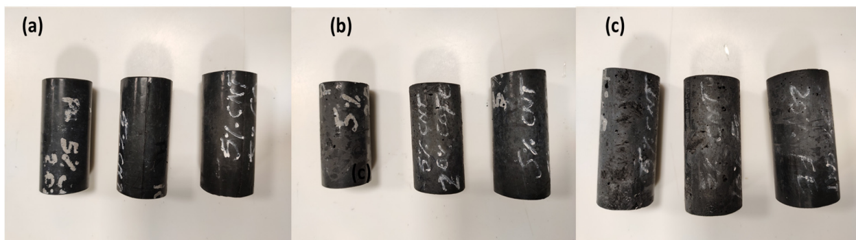
Figure 1. Functionalized samples (a) PU + 5% CNT + (5%, 10%, 20% Co), (b) PU + 5% CNT + (5%, 10%, 20% CoFe), (c) PU + 5% CNT + (5%, 10%, 20% Fe).
