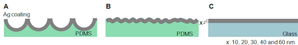
Figure 1. Schematic diagram of the silver nanofilms sputtered on different templates (A) 3D silver nanovoid substrate on PDMS template, (B) 2D silver flat substrate on PDMS template and (C) 2D silver flat substrate on glass slide.
