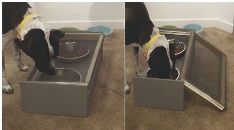
Figure 1. Image of dog with 2-bowl apparatus: a box that contains 2 scales on top of which the food bowls are placed. The scales and bowls were recessed in the circular openings. This prevented the bowls from being accidentally moved off the scale while the dog ate. A removable screen could be slid on top to prevent the dog from accessing the food, but allowed it to see and smell the food options.
