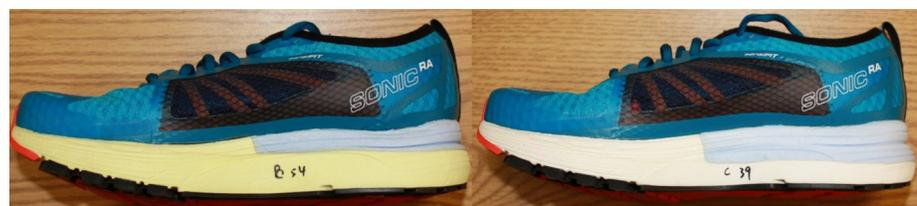
**Fig 1. Testing shoes.** The hard shoe can be seen on the left side, and the soft shoe is on the right side. The overall heel thickness remains the same across shoes, while only the hardness of the EVA foam (yellow/white material) and the thickness of the heel layer (blue material) differed.
