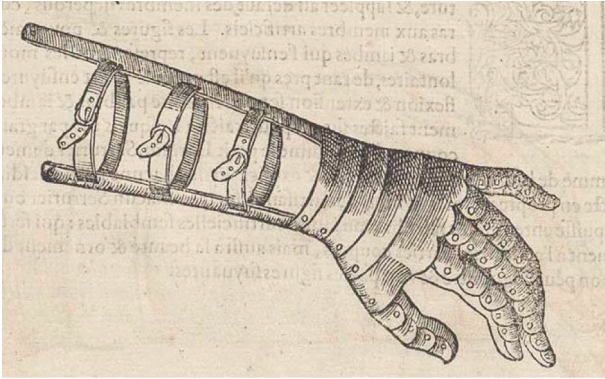
FIGURE 1: Drawing from barber/surgeon Ambroise Paré in the 1500s. The prosthetic hand features buckle straps used to suspend the hand by squeezing the residual forearm skin. Compressive suspension remains the fundamental concept in standard modern prosthetic limbs (reproduced with permission courtesy of the National Library of Medicine. Paré, Ambroise. [Les Oeuvres]. page 916. A Paris: Chez Gabriel Buon, 1585. https://www.nlm.nih.gov/exhibition/historicalanatomies/Images/1200_pixels/ixcxvi.jpg , accessed 7 Feb 2020).
