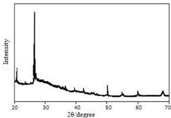
Fig. 2. XRD pattern of porous ceramic membrane.
