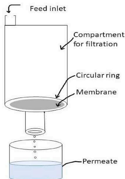
Fig. 1. Experimental setup for filtration test.
