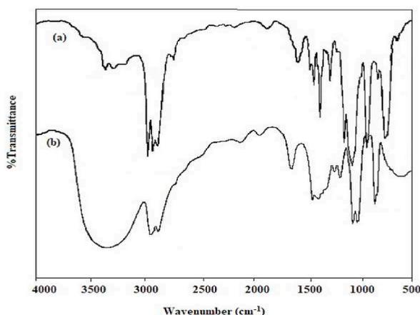
Fig. 5. FTIR spectra of (a) APTES (pure) and (b) Ag coordinated APTES.
