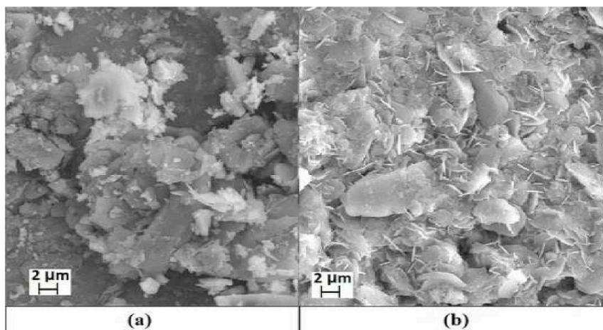
Fig. 4. FESEM images of (a) blank ceramic and (b) Ag-decorated ceramic membrane.
