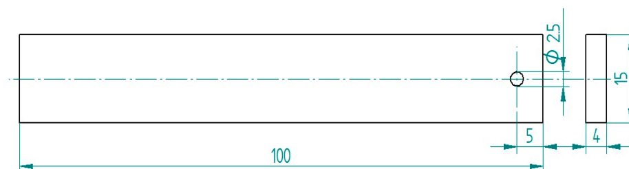
Figure 1. Geometry and dimensions of the adherend.
