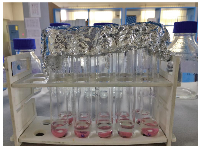
Figs 2: Part of the experimental setup showing enamel samples immersed in demineralization solution
