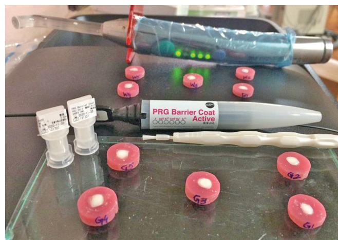
Fig. 1: Experimental setup exhibiting S-PRG barrier coat and enamel samples
