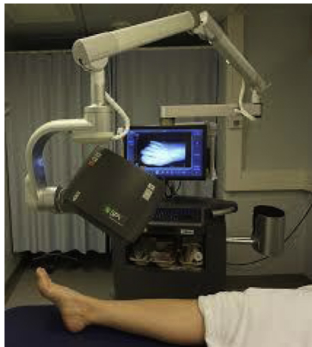
Fig 5. SPY Elite fluorescence imaging system with laser diode and display monitor allows surgeons to evaluate tissue perfusion in real-time without ionizing radiation.
