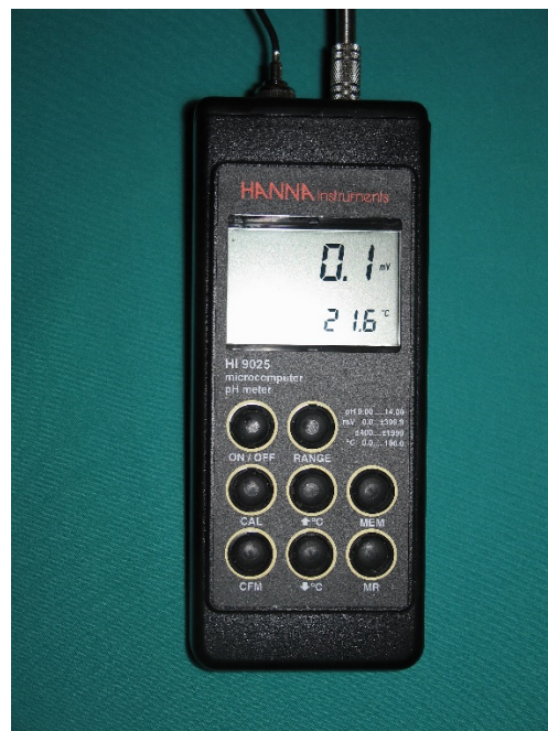
Figure 3. The Hanna waterproof instrument, a heavy-duty pH meter designed to provide accurate laboratory results.
