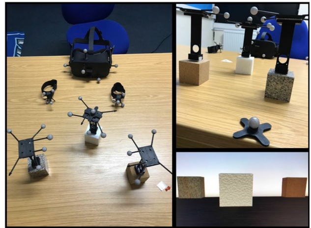
Fig. 3 Tracking Physical Cubes in VR. Note. Participants wore the VR headset and wrist straps to interact with the objects in VR (right). Each physical cube had rigid bodies secured to the top (top right) to allow their movement to correspond to the movement of the replicated VR objects (bottom right)
