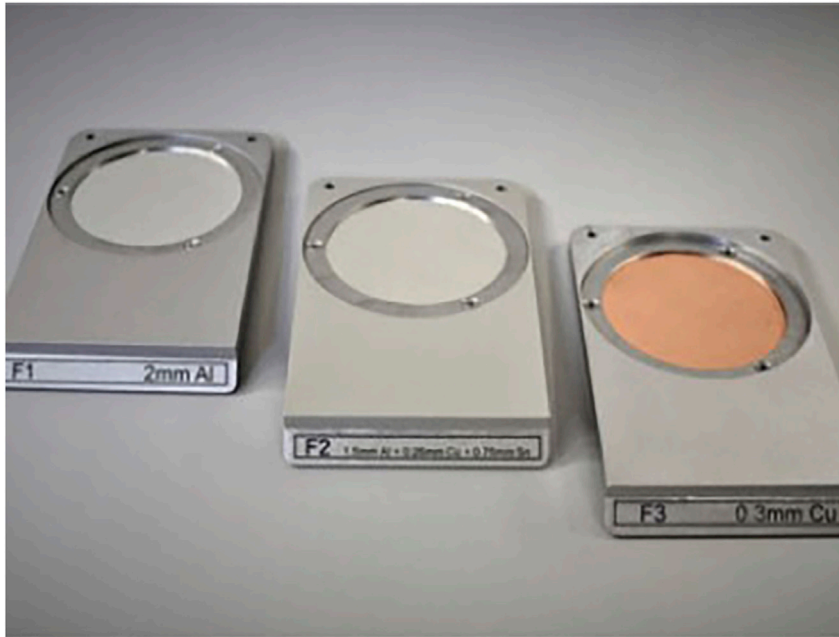
Figure 9. Three types of beam conditioning filters
