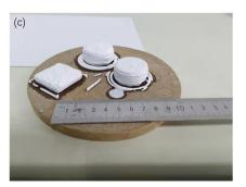
**Figure 2.** Extrusion-based mold printing of alumina ceramics: (**a**) 30 layers of high-hollow pure alumina body; (**b**) alumina green body with carbon fiber added; (**c**) solid pure alumina green bodies with different shapes.
