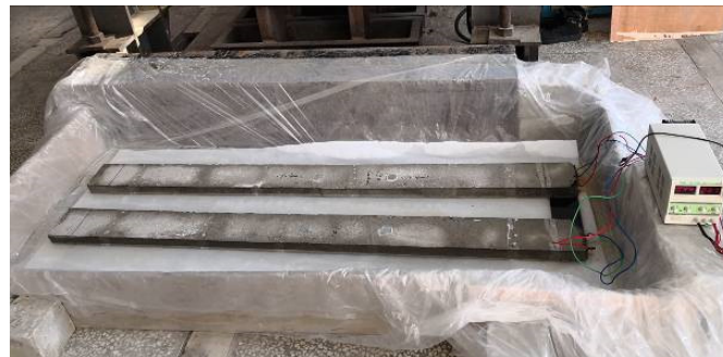
Figure 4. Experimental setup for accelerated steel corrosion.
