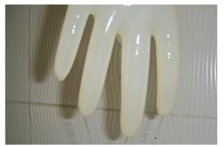
Fig. 1: Identification of perforations by pressurization of the gloves filled with water.
