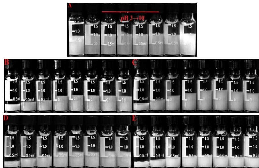
Figure 6. The pH-responsive behavior of hydrogels: (A) Gel 1; (B) Gel 2; (C) Gel 3; (D) Gel 4; (E) Gel 5.
