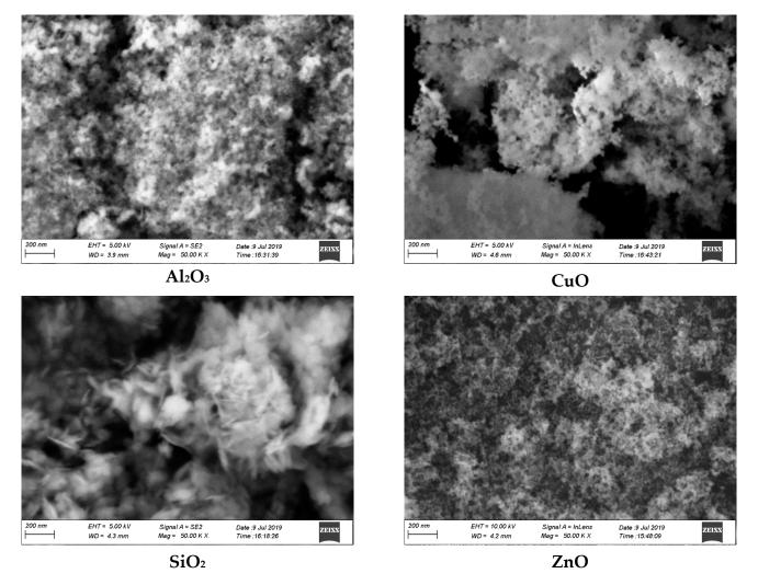
Figure 4. FE-SEM images of different metal oxides nanostructures at the nanoscale of 200 nm.
