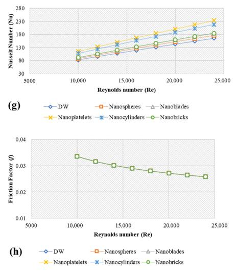
**Figure 6.** Simulation data of average Nusselt numbers and friction factors for different metal oxides and different nanoparticles shape at 4 vol.%, 20 nm, and 293 K; (**a**) Nu-Al<sub>2</sub>O<sub>3</sub>, (**b**) f-Al<sub>2</sub>O<sub>3</sub>, (**c**) Nu-CuO, (**d**) f-CuO, (**e**) Nu-SiO<sub>2</sub>, (**f**) f-SiO<sub>2</sub>, (**g**) Nu-ZnO, (**h**) f-ZnO.
