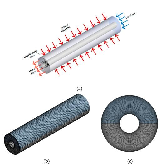
**Figure 1.** (a) Geometric model for the annular heat exchanger; (b,c) Computational meshing domain for 3D and front view of the model.
