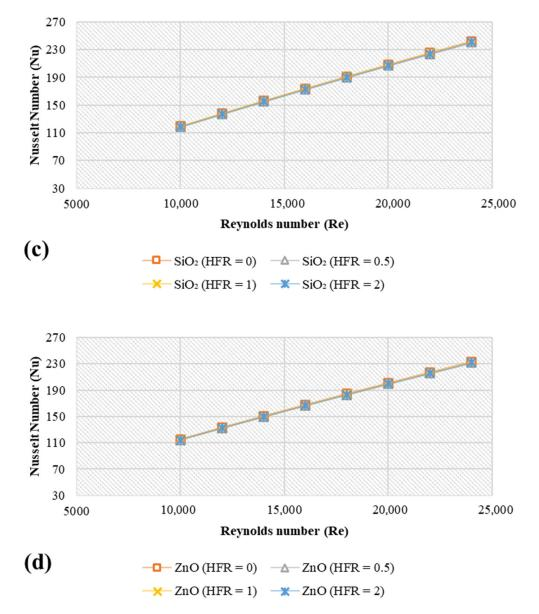
**Figure 7.** Simulation data of average Nusselt number for different metal oxides and different heat flux ratios at 4 vol.%, 20 nm, and 293 K; (**a**) Nanoplatelets -Al<sub>2</sub>O<sub>3</sub>, (**b**) Nanoplatelets -CuO, (**c**) Nanoplatelets -SiO<sub>2</sub>, (**d**) Nanoplatelets -ZnO.
