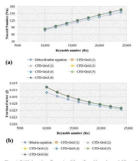
**Figure 2.** Grid Independence Test against different Reynolds numbers and different CFD grid sizes at 293 K; (a) Average Nusselt number, (b) friction factor.
