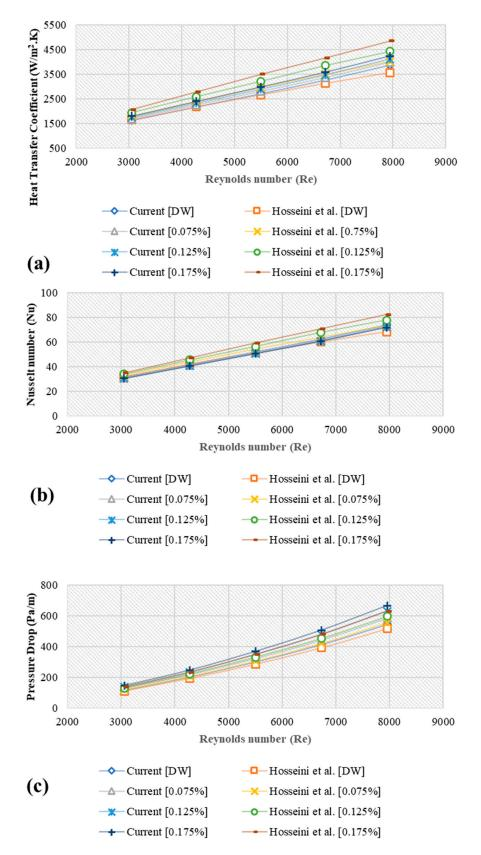
**Figure 3.** Comparison of the results of the current study with those of Hosseini et al. [12]; (**a**) Heat transfer coefficient, (**b**) Nusselt number, (**c**) Pressure loss.
