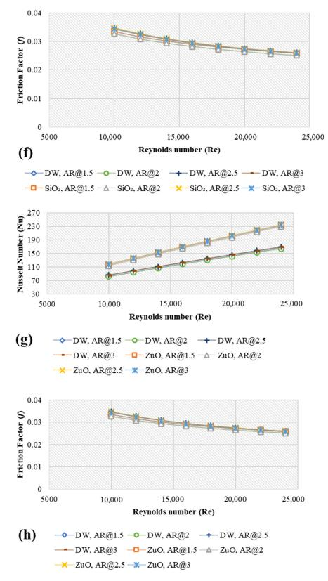
**Figure 9.** Simulation data of average Nusselt number and friction factor for different metal oxides and different aspect ratios at 4 vol.%, 20 nm, and 293 K; (a) Nu-Al<sub>2</sub>O<sub>3</sub>, (b) f-Al<sub>2</sub>O<sub>3</sub>, (c) Nu-CuO, (d) f-CuO, (e) Nu-SiO<sub>2</sub>, (f) f-SiO<sub>2</sub>, (g) Nu-ZnO, (h) f-ZnO.
