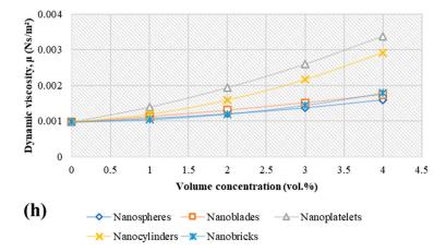
**Figure 5.** Thermal conductivity and dynamic viscosity for different metal oxide nanostructures and different nanoparticles shape at 20 nm and 293 K; (**a**) k-Al<sub>2</sub>O<sub>3</sub>, (**b**)  $\mu$ -Al<sub>2</sub>O<sub>3</sub>, (**c**) k-CuO, (**d**)  $\mu$ -CuO, (**e**) k-SiO<sub>2</sub>, (**f**)  $\mu$ -SiO<sub>2</sub>, (**g**) k-ZnO, (**h**)  $\mu$ -ZnO.
