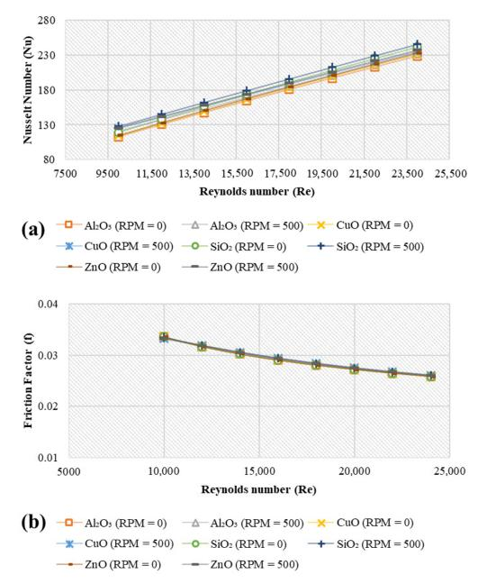
**Figure 8.** Variations of (**a**) average Nusselt number and (**b**) friction factor for different metal oxide nanostructures and different rotation speeds at 4 vol.%, 20 nm, and 293 K.
