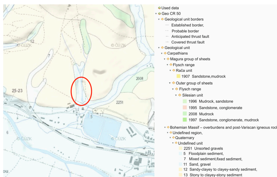
Figure 2. Geological situation of the wider surrounding area on a geological map of CR cut out (1:50,000) with an indicated area of interest.
