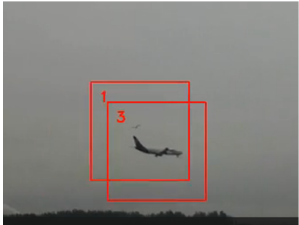
Figure 14. A picture from the monitoring module during the tests—a bird with an airplane in a risk situation. Frame 1 and Frame 3 are centered on the detected bird and the airplane, respectively.
