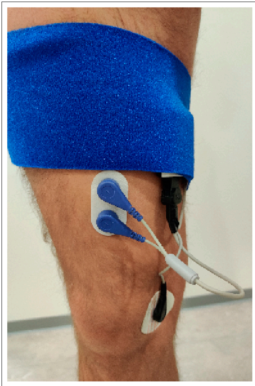
Figure 1. The wireless EMG module placed on the thigh muscles, attached with an elastic ribbon.
