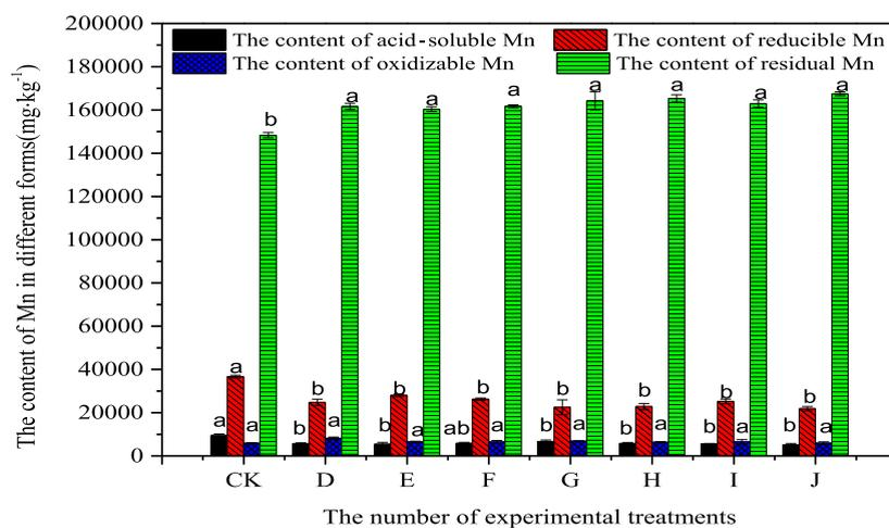
**Figure 6.** Effects of the combined curing agent on the content of different forms of Mn in soil.
