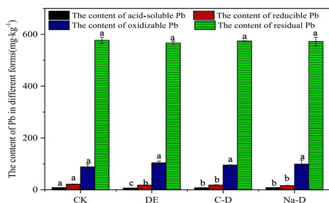
**Figure 3.** Effects of modified diatomites on the contents of Pb in different forms.
