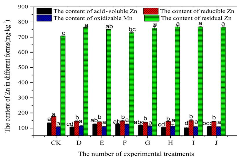
**Figure 8.** Effects of the combined curing agent on the content of different forms of Zn in soil.
