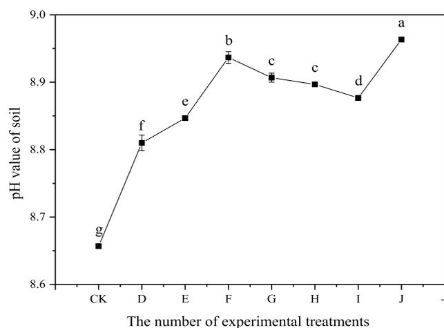
**Figure 5.** Effects of the combined curing agent on the soil pH value.
