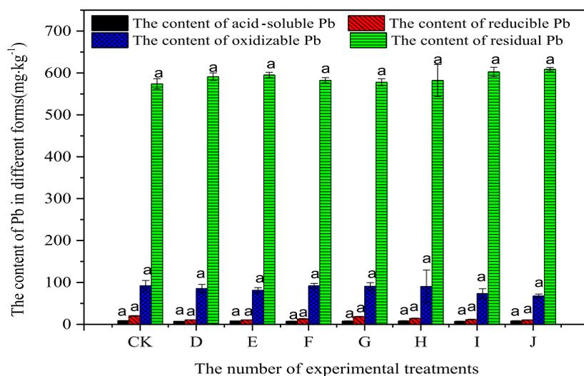
**Figure 7.** Effects of the combined curing agent on the content of different forms of Pb in soil.
