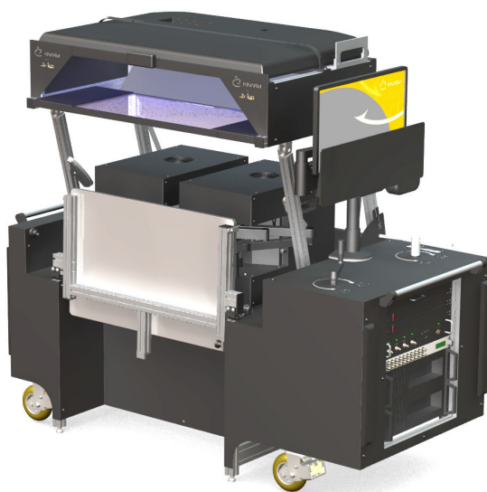
FIGURE 3. KINARM robotic device in collapsed state (Image Courtesy: BKIN Technologies Inc).
