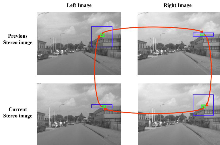
Figure 5. Circle feature matching process. The green boxes represent the matched feature point and the blue boxes represent the search space. The red arrows represent the sequence of the matching process.
