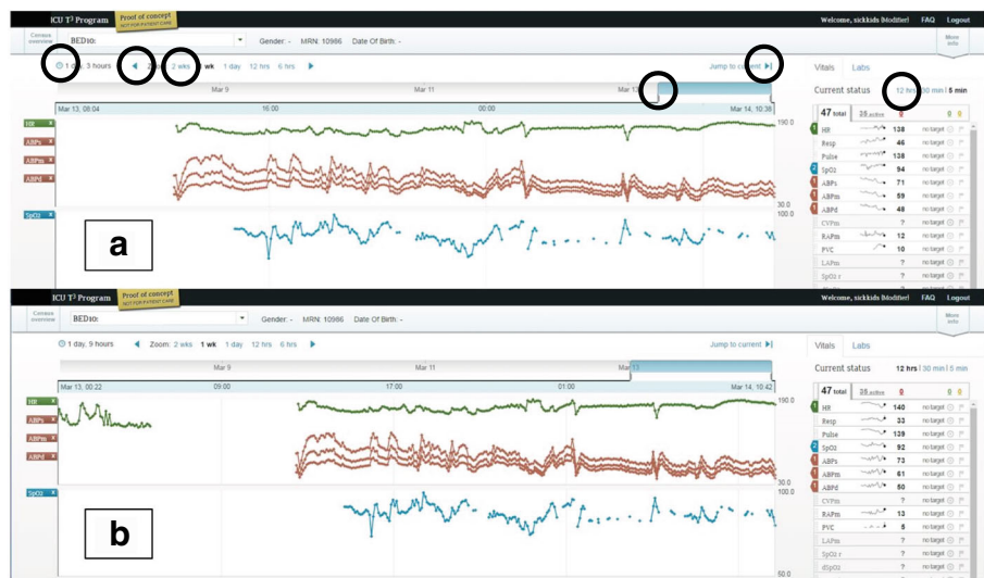
Fig. 5 Usability issue of time manipulation interface. Screenshots of patient view with time manipulation interactive light blue icons, circled on top section, with heart rate, arterial blood pressures, and oxygen saturation data streams. Screenshot a appears to show start and end of data but screenshot b shows the same gap as an interruption in the data streams, signifying the patient was away from the ICU and therefore, was not continuously monitored
