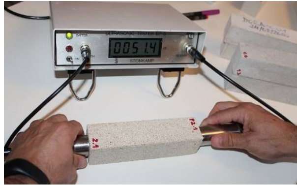
Figure 5. Sample P2.1 (Bateig Beige Hydra) subjected to direct ultrasonic testing.
