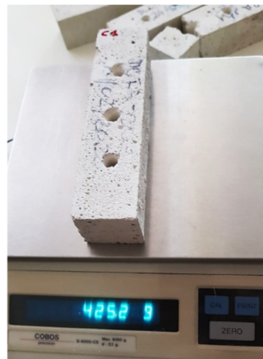
Figure 4. Weighing of the drilled sample in lime mortar.
