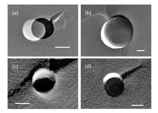
**Figure 1.** Transmission electron microscopy (TEM) images of micro- and nanobubbles (MNBs) in (**a**,**b**) 10 mM and (**c**,**d**) 100 mM NaCl solutions. Each scale bar shows 100 nm. A bubble hole was sometimes covered with thin film (relatively brighter image) formed inside of the hole.
