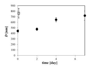
**Figure 5.** Storage time dependence of *D* in 100 mM NaCl solution at 293 K (solid circle). Open squares show *D* in pure water. Error bars are the standard error based on a normal distribution.
