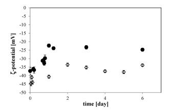
**Figure 7.** Time dependence of the  $\zeta$ -potential of the O<sub>2</sub> MNB solution including 10 mM NaCl (solid circle) and no additives (open diamond). Each error bar shows the standard deviation of the measurement.
