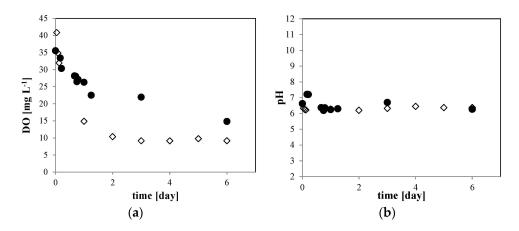
**Figure 6.** Time dependence of (**a**) DO concentration and (**b**) pH of the O<sub>2</sub> MNB in the solution including 0 mM (open diamond) and 10 mM NaCl (solid circle). The measurement uncertainties are within the size of each symbol.
