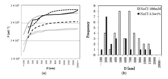
**Figure 3.** (a) The cumulative distributions of *D* in different NaCl concentrations (0 mM: Solid line, 10 mM: larger dashed line, 100 mM: Smaller dashed line, 1 wt %: Dotted line, 3.5 wt %: Double solid line, pure water: thin dotted line). The value at the largest *D* equals the number density *N*. (b) Apparent bubble diameter distributions in 100 mM NaCl solution (coarse dot bar, n = 39), and in 3.5 wt % NaCl solution (fine dot bar, n = 20).
