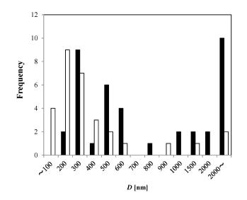
**Figure 2.** Apparent bubble diameter (*D*) observed from TEM-freeze-fracture replica method in 0 mM NaCl solution after 1 h MNB generation (solid bar, n = 39), and in pure water without MNB generation (open bar, n = 31).
