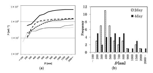
**Figure 4.** (a) Similar to Figure 3 except for 100 mM NaCl solution at various storage periods at 293 K (0 day: thick solid line, 2 days: larger dashed line, 4 days: smaller dashed line, 7 days: thin solid line, pure water: thin dotted line). (b) Apparent bubble diameter distributions in 100 mM NaCl solution 2 days after MNB generation (coarse dot bar, n = 40), and 4 days after MNB generation (fine dot bar, n = 36).
