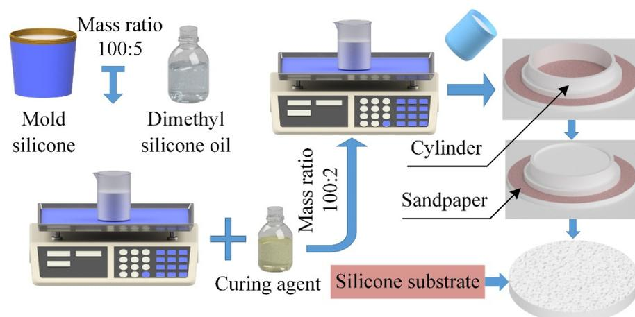
**Figure 2.** The fabricated procession of the adsorption substrate with a rough surface.
