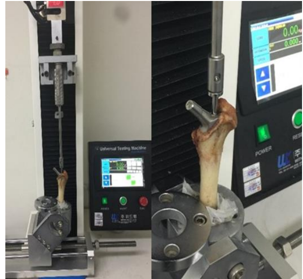
Fig. 1: Images of the yield and failure loading testing of a collarless BFX stem during 5-mm subsidence. After the distal femur was potted in the load frame with polymethyl-methacrylate following osteotomy, the load was applied to the femoral stem parallel to the longitudinal axis of the femur
