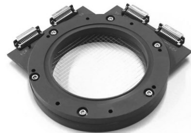
Figure 2. Photograph of the applied wire-mesh sensor with an i.d. of 0.15 m.
