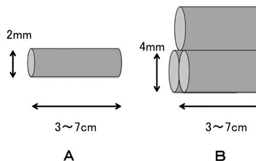
Fig. 5. The illustration shape of control CO<sub>2</sub> absorbent (Sodasorb<sup>®</sup>) (A) and Yabashi lime<sup>®</sup> (B). The shape of Sodasorb<sup>®</sup> is single cylinder. On the contrary, the shape of Yabashi lime<sup>®</sup> is triplet cylinder. Adhesion areas between units in the canister are smaller in Yabashi lime<sup>®</sup> than Sodasorb<sup>®</sup>, so the surface area of Yabashi lime<sup>®</sup> in the canister is larger than Sodasorb<sup>®</sup>.
