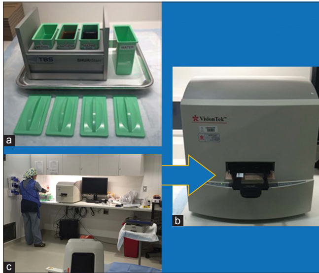
Figure 2: Remote on-site setup (a) The Diff-Quik solution tray used in the interventional radiology suite which is maintained and quality controlled by laboratory medicine. (b) The Sakura VisionTek robotic microscope used in the interventional radiology suite. The arrow designates the slide loading door with stable tray mechanism which is simple and not prone to breakage or jamming. (c) Proximity of the Sakura VisionTek, situated adjacent to the interventional radiology procedure table
