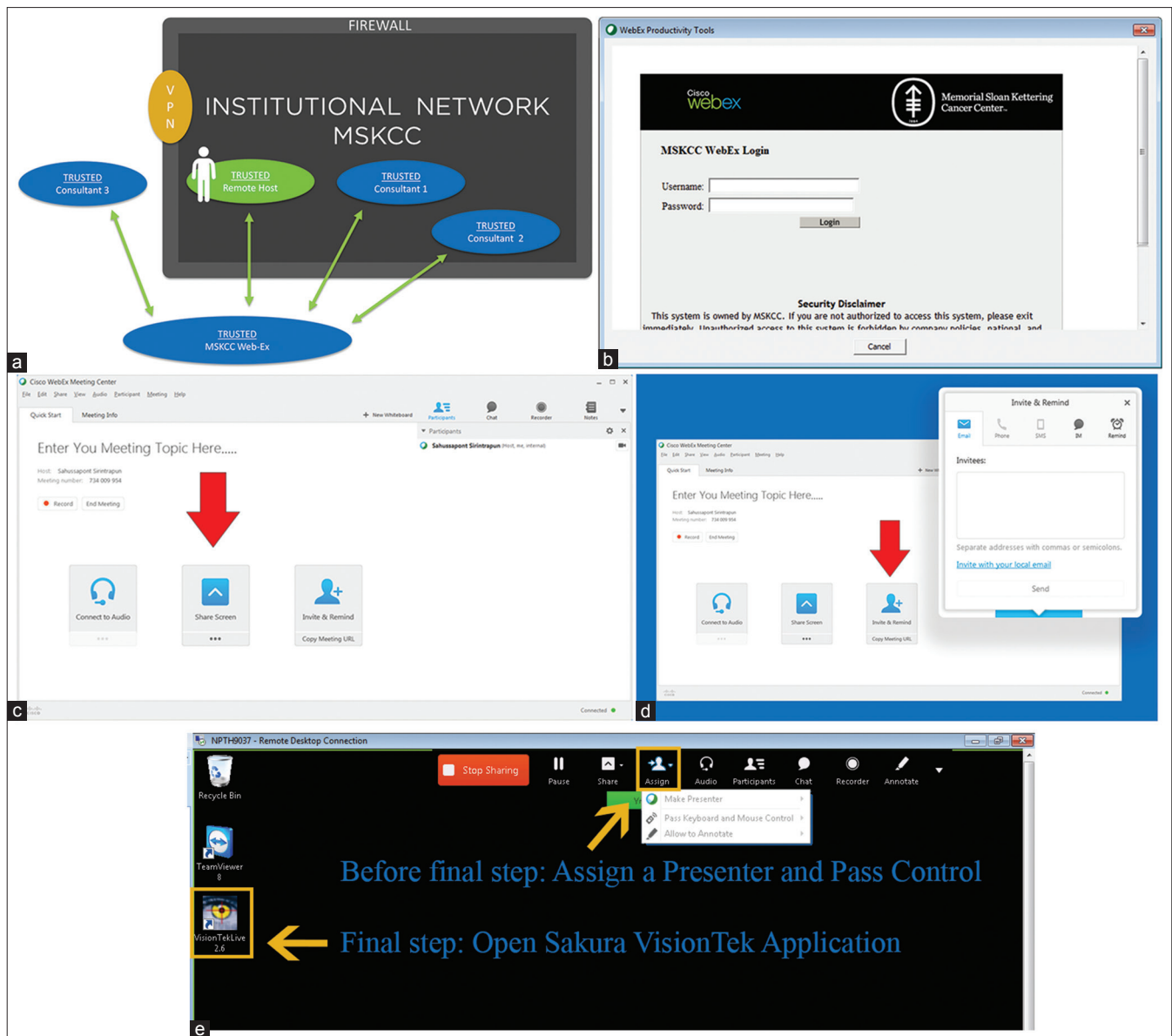
Figure 7: The WebEx external desktop sharing solution (a) overall schematic of the Memorial Sloan-Kettering dedicated WebEx architecture. WebEx can bypass the normal VPN procedures to access internal workstations behind the firewall, from external sources. Images from the Sakura VisionTek desktop application can then be shared with multiple parties both internal and external to our institutional firewall along with desktop control. The human figure represents the need for a person at the remote satellite site to initiate the WebEx session or another person off-site using remote desktop to login the workstation and then initiate the WebEx session by performing the WebEx login and password procedure. (b) screenshot of the Web-Ex login with the input of username and password. For first time logins, a Web-Ex plug-in is required per workstation that can cause further delays. (c) screenshot of host setup with screen share, once logged in. Each workstation must be manually configured for Voice over Internet Protocol if the default phone option is not desired. (d) screenshot of the invitation procedure for consultants, which often requires knowledge of the consultant’s email. On the consultant side, email notifications allow the consultant to click and download the appropriate plugins, for viewing the Web-Ex session. (e) screenshot of the top panel on the screen for requesting or passing desktop sharing control; steps required all before starting the Sakura VisionTek desktop application
