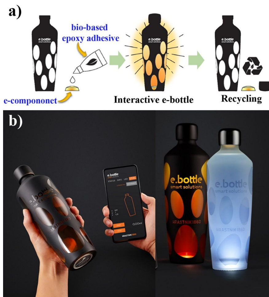
Figure 10. Schematic presentation of the development of an innovative glass e-bottle using the prepared bio-epoxy adhesive (a) and pictures of the final product (b).
