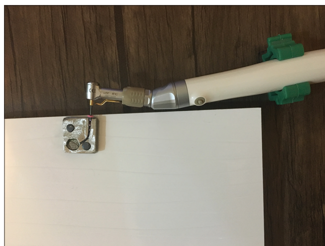
Figure 2: A dental handpiece mounted on the block with the instrument inserted in an artificial root canal.
