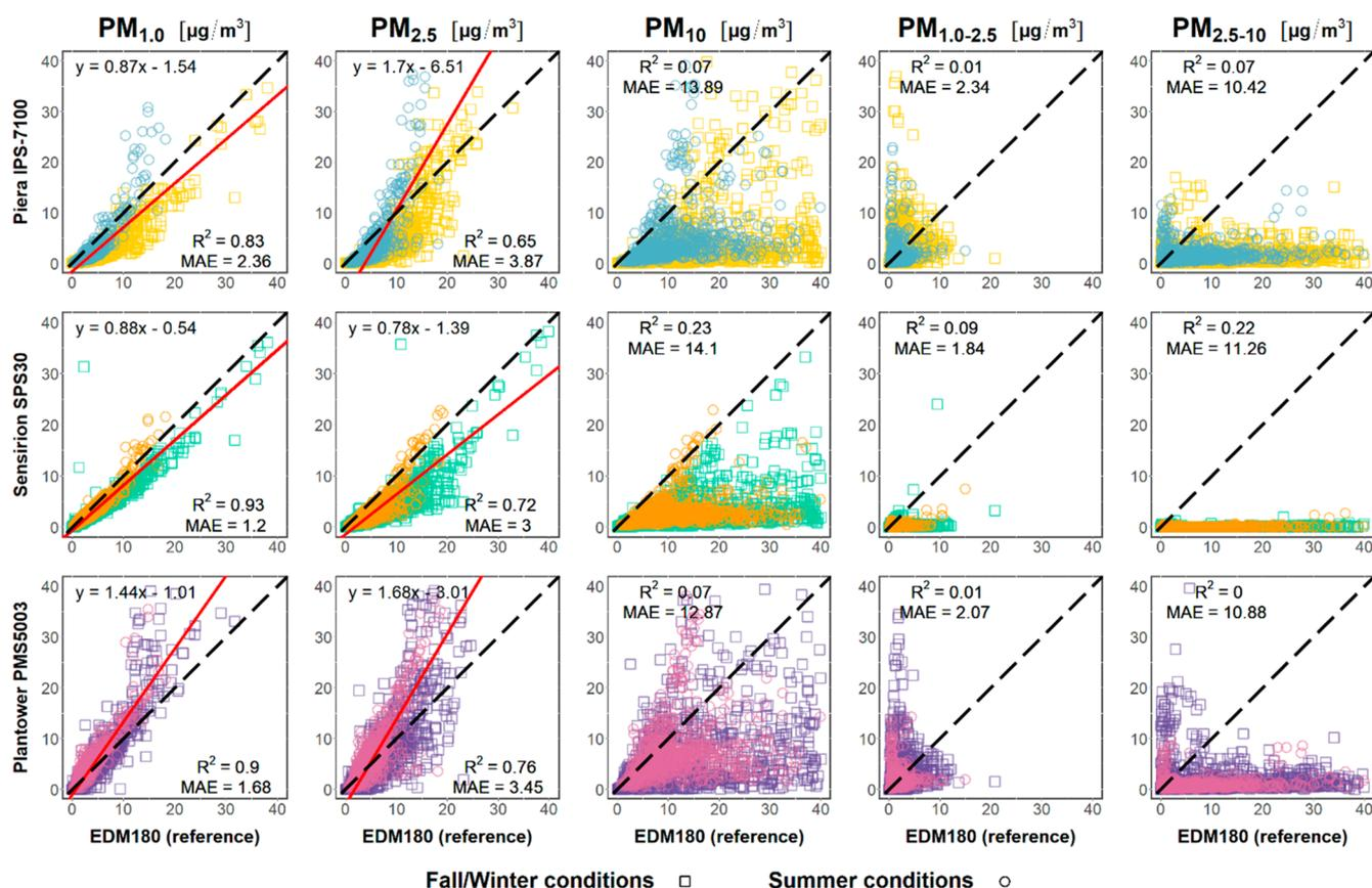
**Figure 2.** Regression plots of low-cost sensor PM estimates versus the EDM180 reference measurements. Dashed black lines are identity (1:1) lines, and continuous red lines are the lines of best fit (for models that complied with linear regression assumptions). All the hourly averages ( $n = 1763$ ) were used to compute the regression models, but some points are not shown in the plots due to the axes ranges.
