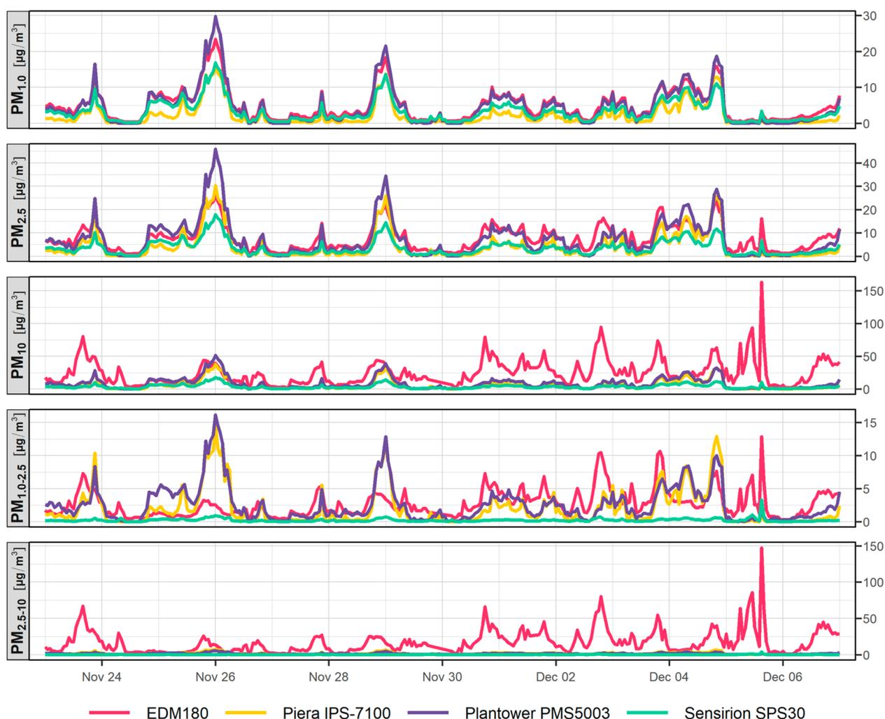
**Figure 1.** Time series graph of PM concentrations (cumulative and differential). A subset composed of the first 14 days of the fall/winter period is shown to improve readability. A similar plot for the summer period is available in the SI (Figure S7).
