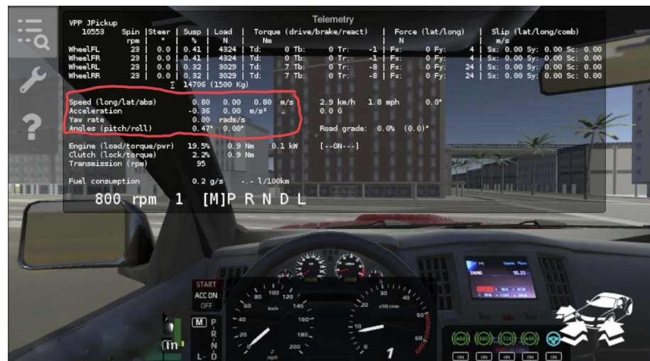
Figure 4. Vehicle Physics simulator. In the red box, the data that we collected during the simulation.
