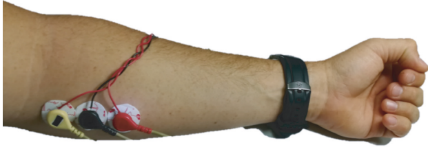
FIGURE 6: Location of the electrodes on the long palmar muscle for simultaneous connection of the proposed system and the Shimmer commercial system.
