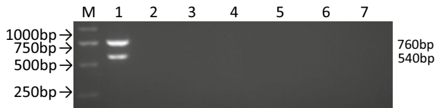
Fig. 1 The specificity of the one-step dPCR assay. M: DL2000 DNA Marker; 1: CDV, CCoV; 2: CPV; 3: ICHV; 4: CPIV; 5: CHV; 6: E. coli ; 7: Negative control
