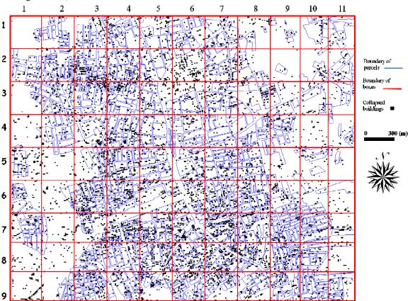
Figure 5. Blocks overlaid on the difference image (black: damaged areas, white: non-damaged areas)
