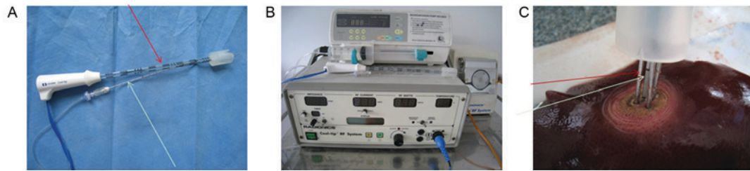
Figure 1. RF applicator. The instrument comprises (A) RF probes and (B) an RF generator. (C) A high-resolution image of 3 cool-tip electrodes (red arrow) and 1 perfused hypertonic-saline-augmented needle (white arrow) outlining the infusion system. RF, radiofrequency.
