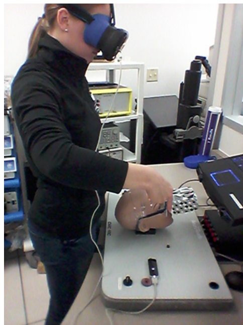
Fig. 9 Participant using the NeuroTouch system, in the process of targeting – moving toward the anterior horn of a ventricle
